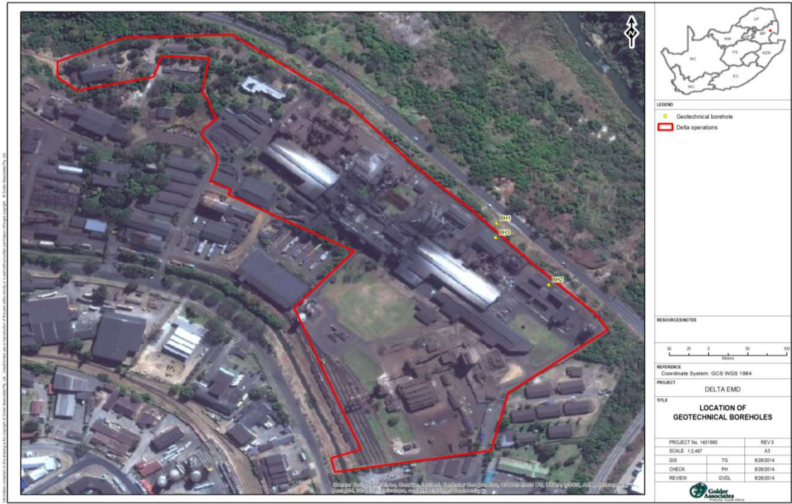
Figure 5: Borehole Location Drawing
