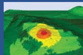
Isopleth diagrams help indicate noise levels from a projected wind turbine location
