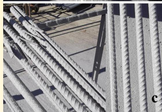
Fig. 1. a) Spray-application of polyurea coating, b) polyurea coated split sets, c) polyurea coated rebars
