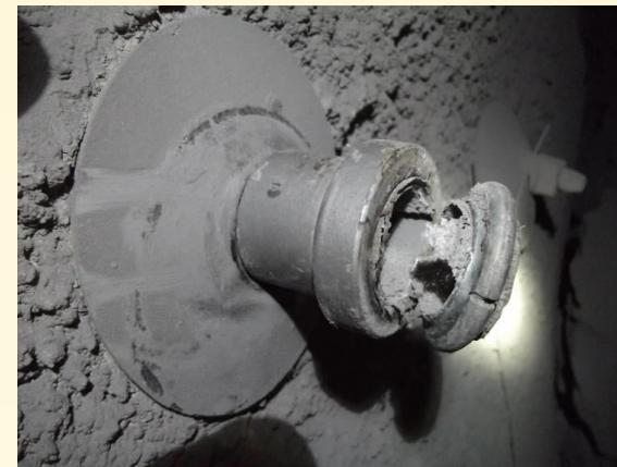
Fig. 2. Example of broken steel of split set with polyurea coating after a completed pull test
