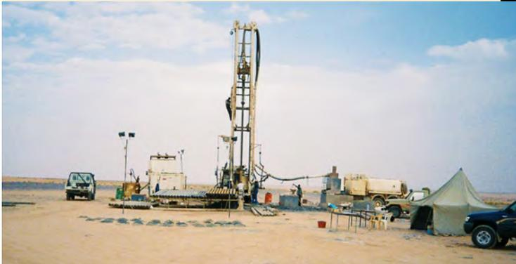
Golder was retained to carry out geological due diligence and an initial resource evaluation for a proposed limestone quarry for cement production in the Middle East. The work program included a geological assessment through drilling and sampling as well as the creation of a geological model for the purpose of determining an accurate resource estimate for the site prior to purchase. The work was used by the client to make an informed decision regarding the value of the purchase.
